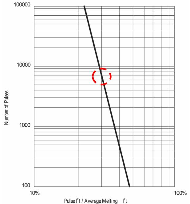
Figure 6. Pulse I<sup>2</sup>t capacity [6].
