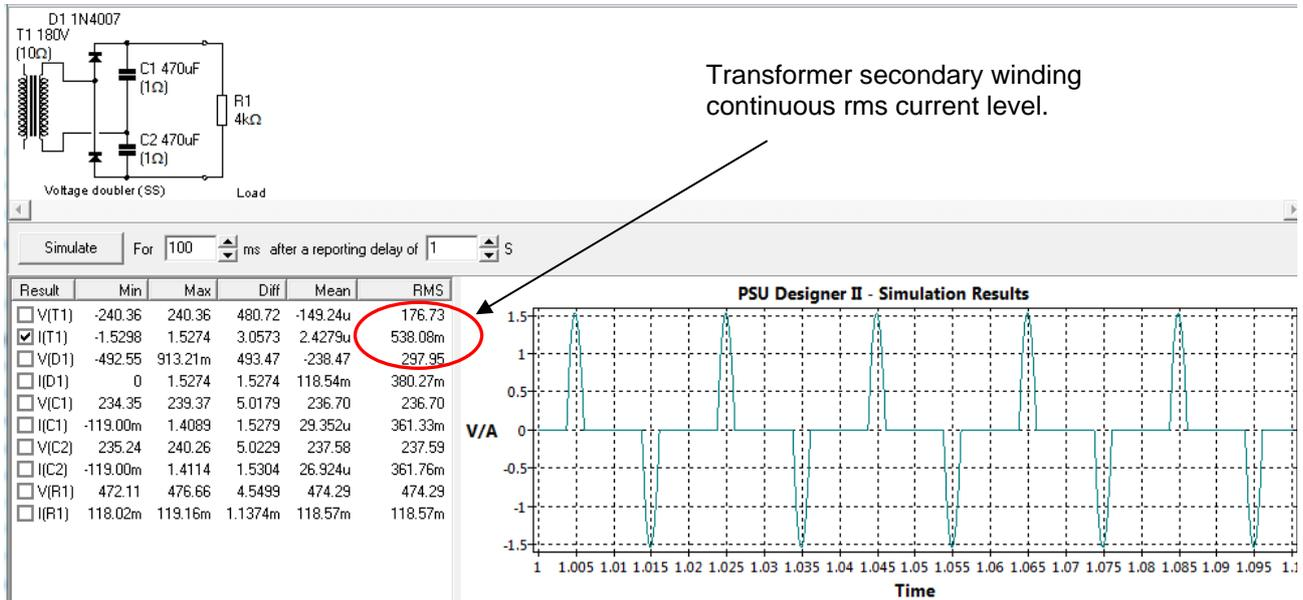
Figure 3. PSUD2 screen showing doubler power supply and simulated operating levels.
