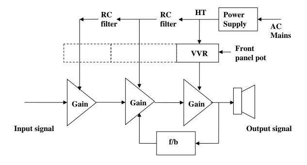
Most amps and combos generate a pleasing sound character when the volume is raised to the point where overdrive and other higher level distortions become significant. But not everyone is enamoured by the sound levels of a cranked amp. With this in mind, an increasing number of amps are being modified to include VVR (also referred to as 'power scaling'). A variety of kits of parts are available, and the technique is well within reach of those who are happy to electrically modify an amp.
