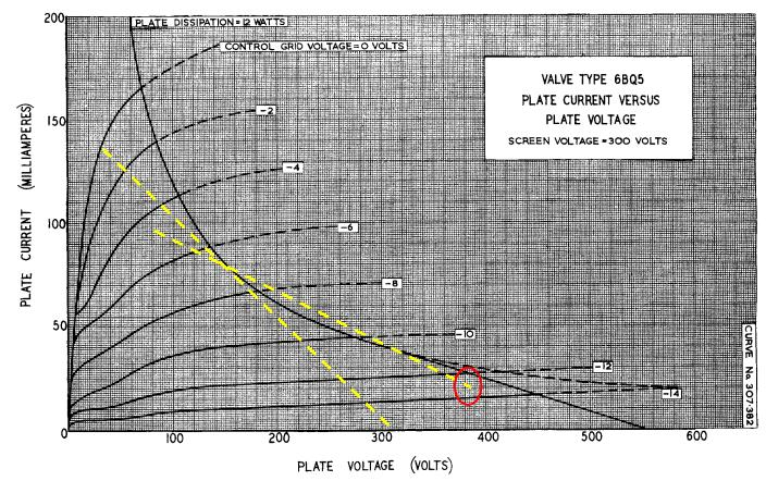
Now if we use VVR to reduce the idle voltage down to say 250V, then the loadline looks like the following graphic, which uses characteristic curves for screen voltage of 200V. Note that sagging of the HT voltage is less in this case as signal levels are lower, so the loadline assumes a sagged voltage level of 200V is available for high loads. Loading impedances don't change.
