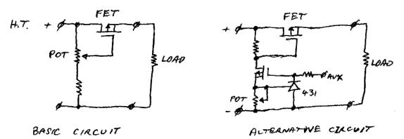
This technique also allows multiple main FETs, placed in series, to equally share the dropped voltage between the HT supply and the amp stage, and for these FETs to be controlled with a single pot. And this technique also provides a convenient point to interface other control signals, if needed.
