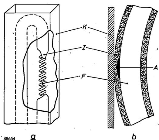
Fig. 7. a) Indirectly heated oxide cathode. K nickel cathode tube, F tungsten heater, surrounded by an insulating layer of alumina I.
