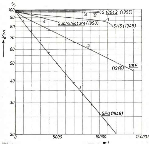
Fig. 2. The percentage  $S/S_0$ , on logarithmic scale, as a function of time  $t$ , for life tests on various types of valve. The curves 1...5 have been taken from published sources<sup>1)...</sup>; the valve type and the year of publication of the curves are given in each case. The data for curves 5A and B were obtained from a test made with the cooperation of the Netherlands Post Office.
