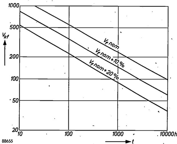
Fig. 8. Potential  $V_{kf}$  (heater positive with respect to cathode) as a function of the time  $t$  in which 1% of the valves show heater-cathode short-circuits, at nominal heater voltage  $V_{f\text{ nom}}$  (heater temperature 1080 °C) and at 10% and 20% higher heater voltages. Provisional curves only, obtained by extrapolation of accelerated tests.)
