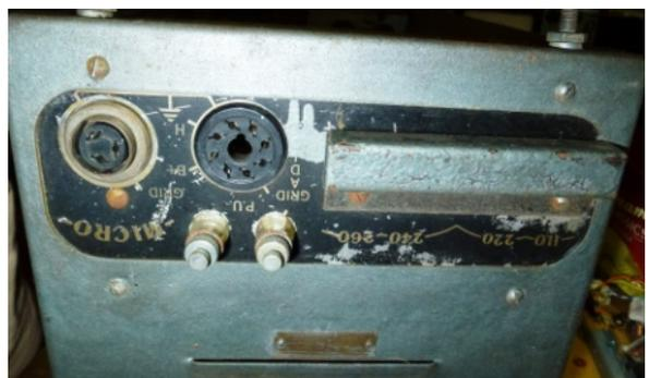
Older PA with hazardous terminals; hardened and crumbling rubberized wire insulation; & optional DC powering with vibrator. Circa mid 1940's Australian Sound Systems A13.
