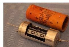
Modern e-caps are much smaller than vintage caps, so confirm the ripple current rating of a new cap is
