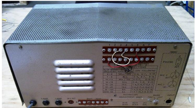
Rear of AWA PA1001; multiple speaker screw terminals; bass cut switch. Inputs on side panel.
