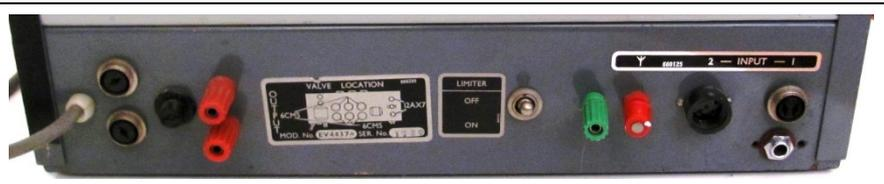
Typical looking late Philips PA and rear connections. Layout & input labels. 100V line output only.
