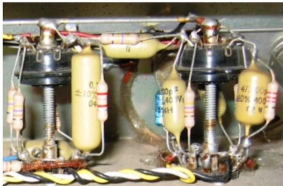
Some valve base spigots have a 'tree' attachment to simplify the local connection of parts without having to use connecting wire to nearby tag boards. The photo shows an example of tree spigots.
