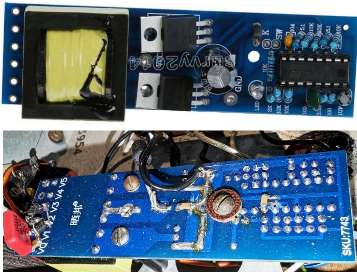
Figure 39. '150W' inverter module with added rectifier/filter.
