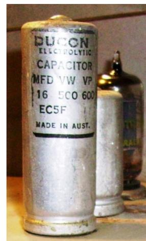
The IEC 60384-4 surge voltage test relates to an example 1k $\Omega$  resistance in series with a 100uF e-cap, which is likely not valid for the first filter capacitor location, but may exist for screen and preamp type filter capacitor locations that are buffered by feed resistance.
