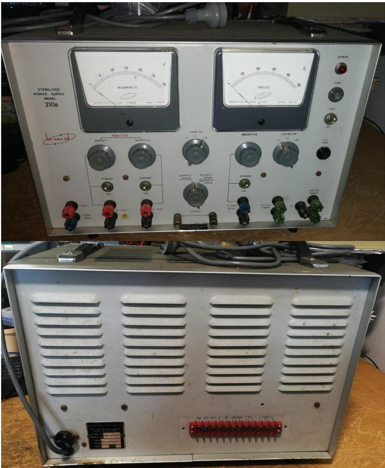
2x 500Vdc regulated outputs (300mA, or 180+150mA); 1x 250V regulated 50mA; 2x 6V3 5A. Separate voltage and current meters. This unit S.N.4405 appears to be an Iss.1 from 8/65 as it doesn't include the Iss.2 mods from 4/67 or Iss.3 mods from 7/68, and at least 3 other circuitry differences so far to the Iss.4 schematic. The part date-codes indicate earliest manufacture from July 1966, which is consistent.
