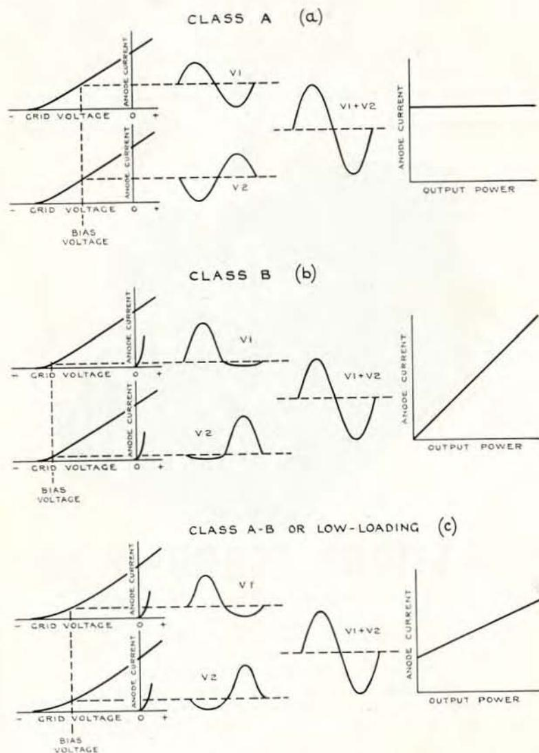
Fig. 4. Illustrating the operation of push-pull output valves when working in Class A, Class B and Class A—B (low loading). The transformer design and grid-bias are the factors governing the manner in which the valves function.
