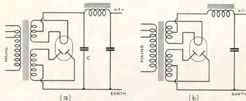
Fig. 10. (a) illustrates the usual condenser input to the smoothing filter, while (b) shows the choke input circuit that has to be used where good H.T. regulation is essential.
