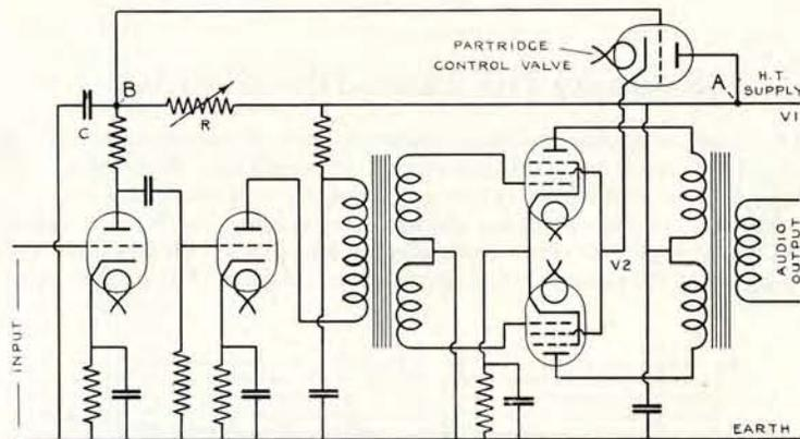
Fig. 5. The Partridge Control Circuit. Invented and provisionally patented by N. Partridge, B.Sc., A.M.I.E.E., patent rights purchased and controlled by The Mullard Radio Valve Co., Ltd.
