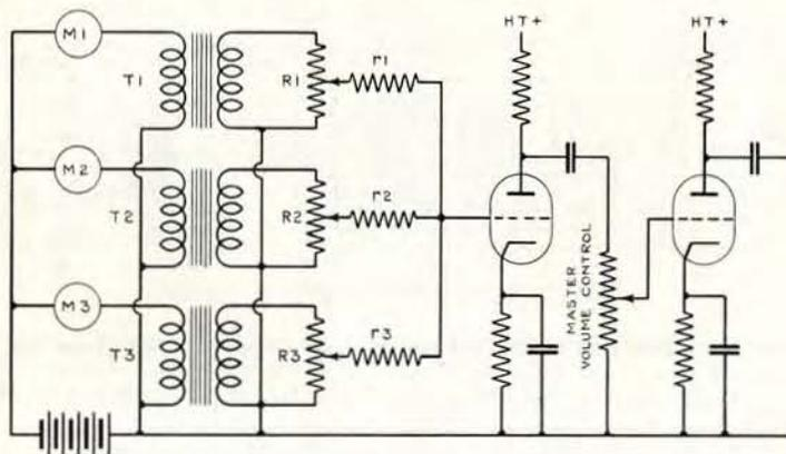
Fig. 14. Mixing three high sensitivity microphones. Note the master volume control, the use of which is explained in the text.  $R_1$ ,  $R_2$ ,  $R_3$ ,  $r_1$ ,  $r_2$ ,  $r_3$  are all 250,000 ohms.
