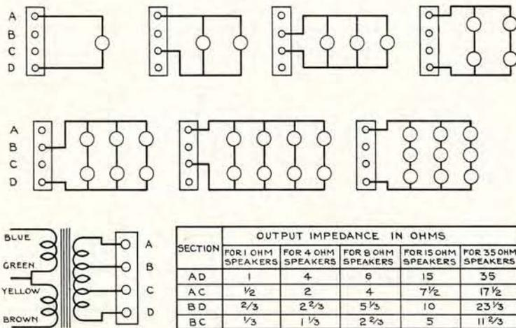
Fig. 20. Method of connecting the Parallel Type Partridge Output Transformer. This is recommended where short lines are used and where a single speaker is required more frequently than a number of speakers.
