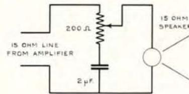
Fig. 18. A tone compensated circuit for controlling the volume of individual speakers.
