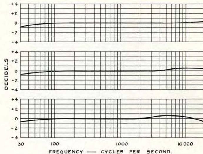
Fig. 23. Response curves of the Partridge Single-Stage Pre-Amplifier with 15, 30 and 45 yards of screened flex. The 15 yard curve is at the top and that for 45 yards at the bottom.
