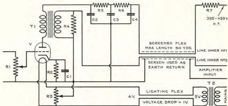
Fig. 22. Partridge Single-Stage Pre-Amplifier. Note the method of using the screened flex and the L.T. line.
