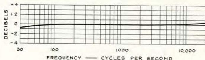
Fig. 7. Response curve of the Partridge Intervalve Transformer Type IV240.
