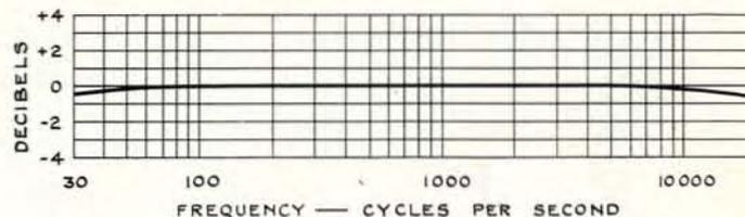
Fig. 17. A typical response curve of a Partridge Output Transformer.
