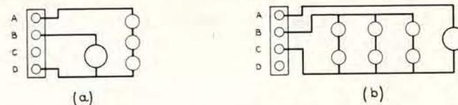
Fig. 21. The speaker connected across B—D in circuit (a) and also that across A—C in circuit (b) receives six times the power taken by each of the other speakers.
