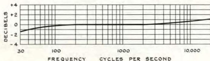
Fig. 6. Response curve of the Partridge Intervalve Transformer Type IV60.
