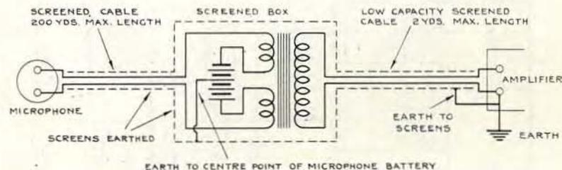
Fig. 13. The correct method of connecting and screening a microphone line.
