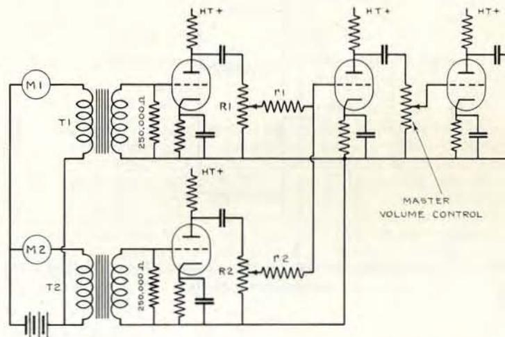
Fig. 15. This circuit is suitable for mixing low sensitivity microphones. Extra input channels can be added if desired.  $R_1$ ,  $R_2$ ,  $r_1$ ,  $r_2$  are all 250,000 ohms.
