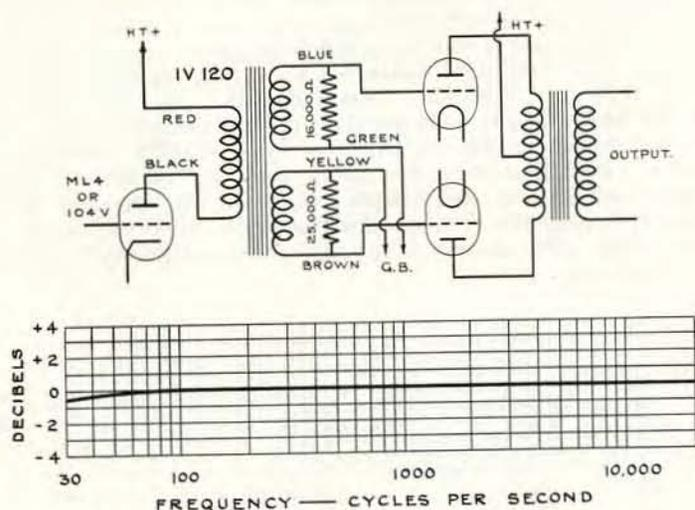
Fig. 8. Showing the circuit arrangement and response curve of the Partridge Intervalve Transformer Type IV120. This is probably the most perfect coupling obtainable.
