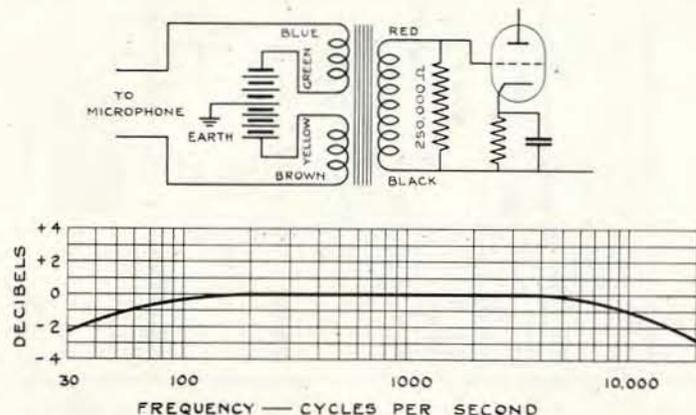
Fig. 12. The circuit diagram and response curve of the Partridge Microphone Transformers Types M250/350 and M400/600. Note that the primary is split into two equal sections so that the line may be balanced with respect to earth.
