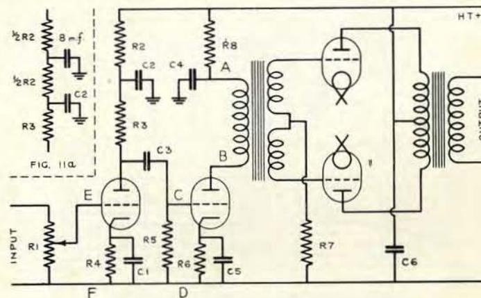
Fig. 11. A typical amplifier circuit used in the text to illustrate how to locate and remove hum.
