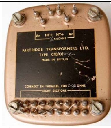
T/CFB with 43% UL connections
