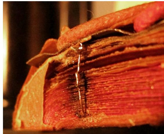
**Figure 11. Repairable fault in output transformer.**
