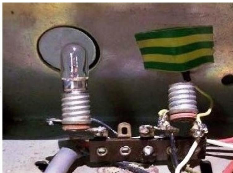
Figure 8. Goldentone made their OT secondary loading resistor into the RYTHYM LIGHT 'feature' on the front panel, which provides about 10% loading, and a touch of non-linear compression due to resistance change.
