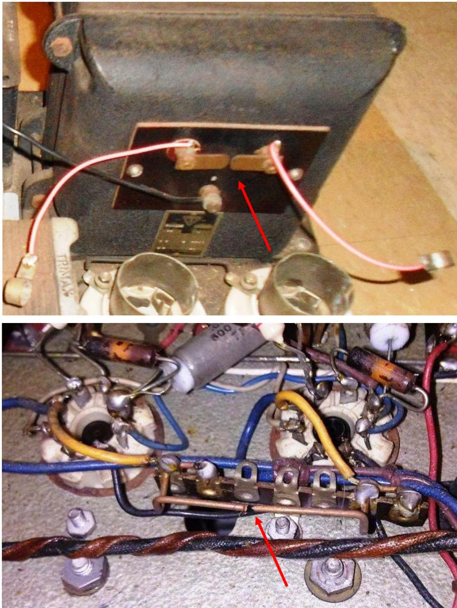
**Figure 6. Examples of spark gap placed from plate-to-plate.**
