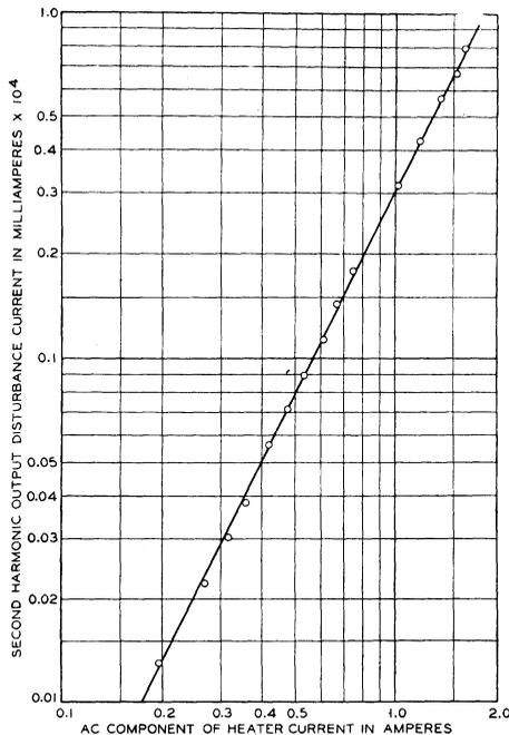
Fig. 7—Second harmonic output disturbance current produced by the magnetic field as a function of the alternating-current component in the heater.
