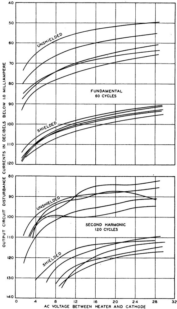
Fig. 5—Disturbance current measurements on shielded and unshielded tubes with the circuit of Fig. 4.
