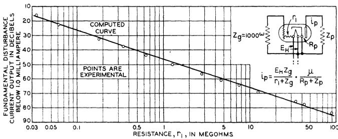
Fig. 9—Fundamental disturbance output current as a function of the grid-to-heater resistance.
