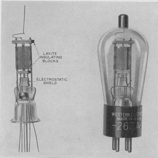
Fig. 10—No. 262A mount and completed tube.
