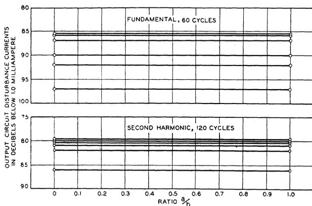
Fig. 3—Disturbance currents in indirectly heated cathode triodes having shields to reduce the electric field of the heater in the cathode-plate space.
