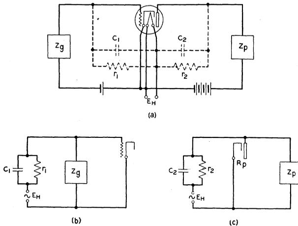
Fig. 8—Diagrams of disturbance current circuits between heater and grid and heater and plate.
