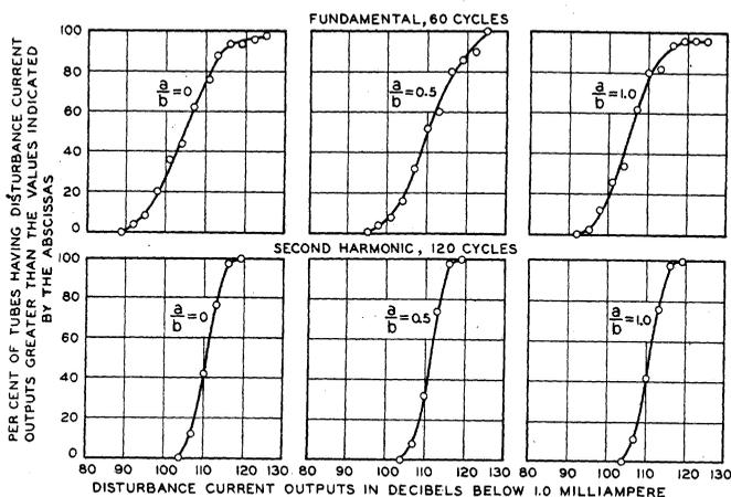
Fig. 12—Distribution of disturbance output currents in a representative number of No. 262A tubes picked at random.
