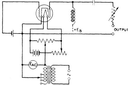
Fig. 4—Circuit for the study of the electrostatic effect in the presence of large disturbance outputs due to the magnetic field.
