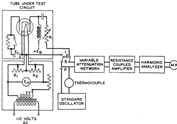
Fig. 1—Schematic diagram of disturbance current measuring circuit.
