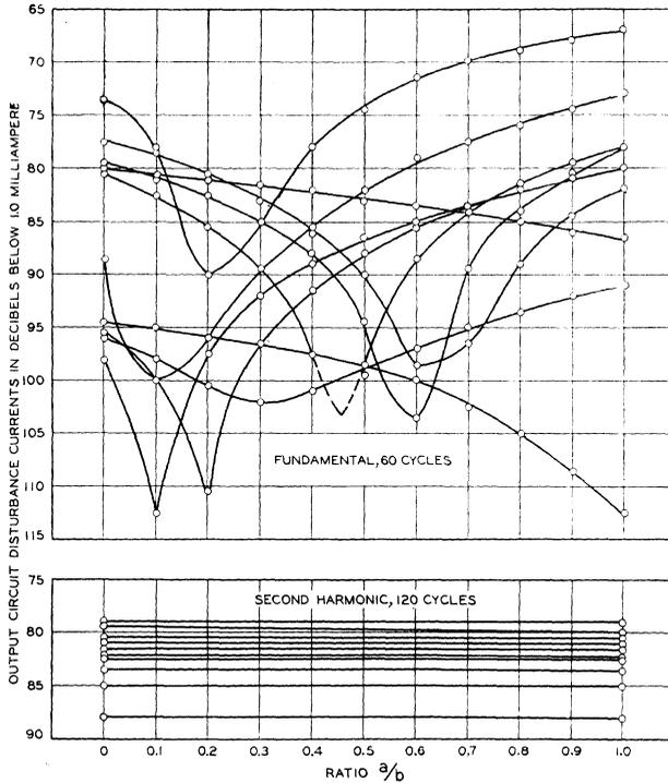
Fig. 2—Disturbance currents in typical indirectly heated cathode triodes used for radio reception.
