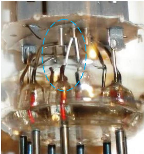
Figure 5. Heater loop entering cathode in 12AX7.
