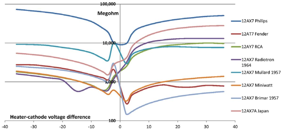
Figure 4. 12AX7 heater-cathode resistance.
