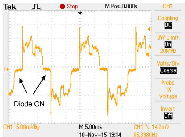
**Figure 30. Capacitive coupled signal from wiring**
