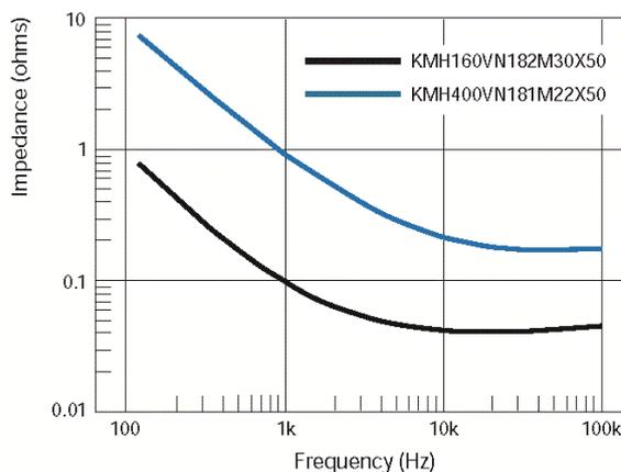
Figure 18. Capacitor impedance.
