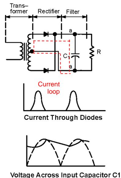
Figure 19. Capacitor input filter.
