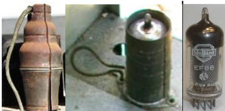
Figure 33. External and internal shields.
