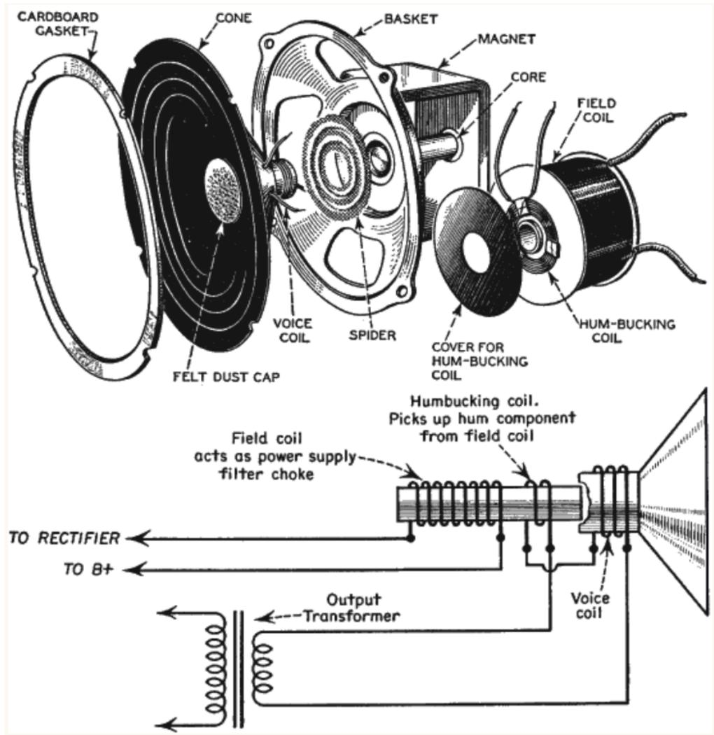
Figure 12. Speaker with electromagnet and hum-bucking coil.
