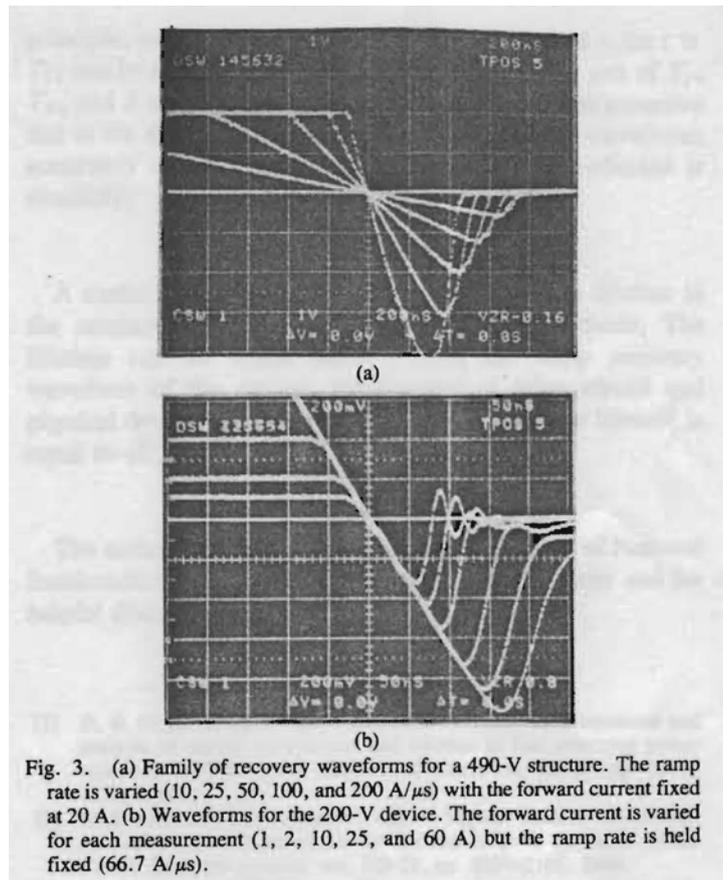
Fig. 3. (a) Family of recovery waveforms for a 490-V structure. The ramp rate is varied (10, 25, 50, 100, and 200 A/ $\mu$ s) with the forward current fixed at 20 A. (b) Waveforms for the 200-V device. The forward current is varied for each measurement (1, 2, 10, 25, and 60 A) but the ramp rate is held fixed (66.7 A/ $\mu$ s).
