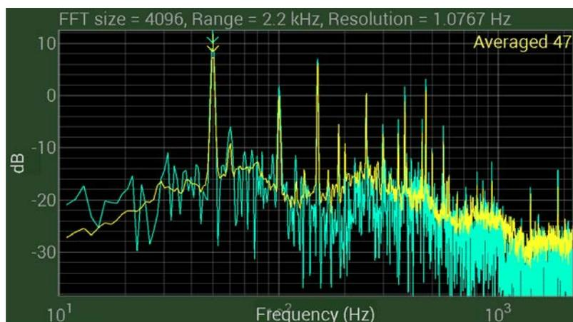
Figure 35. Audible hum measured on Android phone.
