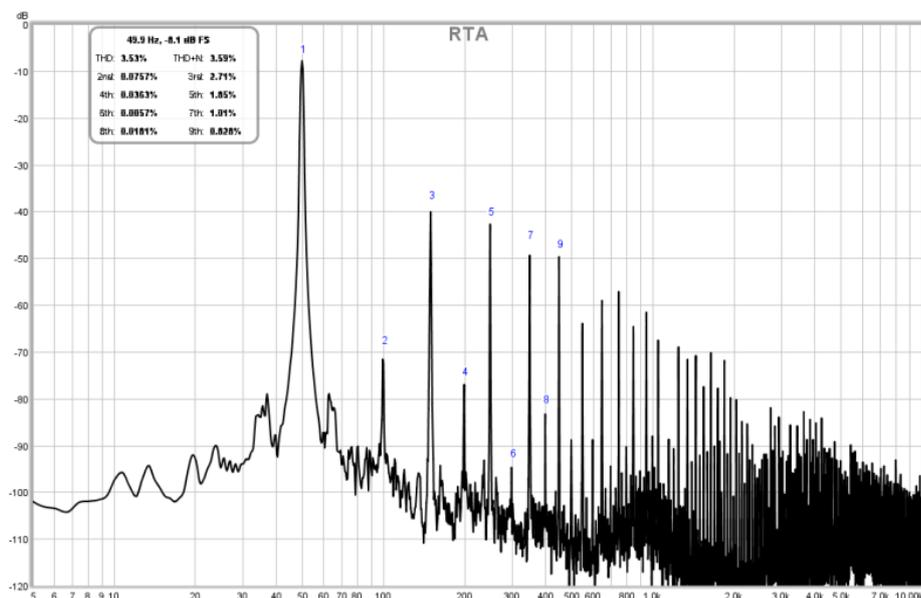
Figure 22. Mains voltage spectrum using REW V5.1 software.
