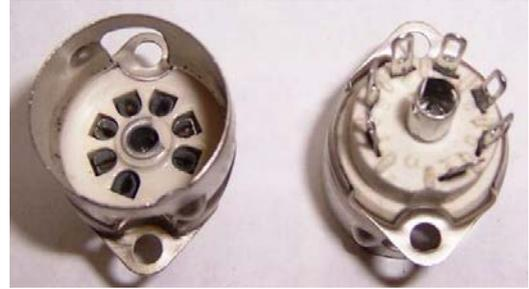
Figure 9. Socket with spigot & collar
