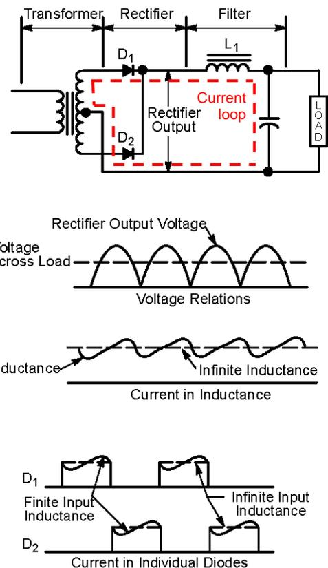
Figure 17 Choke input filter. [Rectifier applications handbook HB214/D]
