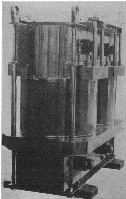
**Fig. 4. A complete 7<sup>1</sup>/<sub>2</sub> kw third stage transformer**
