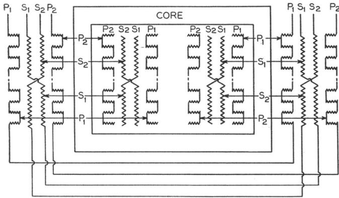
**Fig. 3. Schematic diagram showing arrangement of windings in 7<sup>1</sup>/<sub>2</sub> kw third stage transformers**
