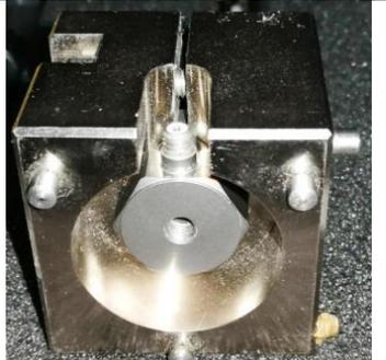
A cylindrical metal accelerometer mounted on a square metal mounting block. The accelerometer has a central silver-colored tip.                                                                              |
