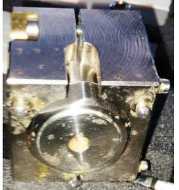
A cylindrical metal accelerometer mounted on a square metal mounting block. The accelerometer has a central gold-colored tip.                                                                                 |
