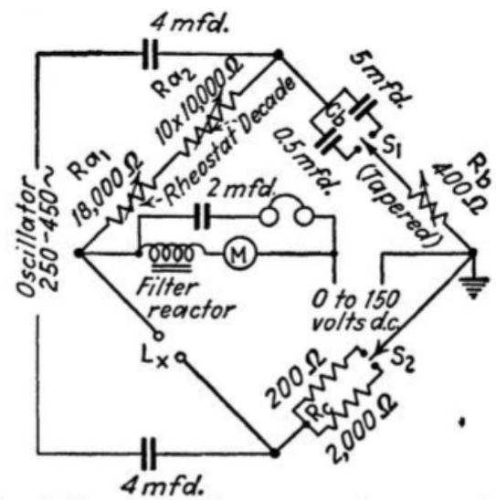
Fig. 39.—Hay bridge arranged to measure incremental inductance.
