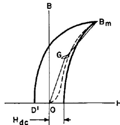
As the measurement scheme uses average (RMS) measures of choke AC voltage and AC current, any detail of the change in incremental inductance is lost unless multiple measurements are made with small AC level as DC is step increased. Also care is required when applying high levels of AC voltage.
