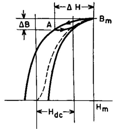
application. With respect to what the choke core experiences for this application, the graph on the right shows the choke core magnetised with the DC magnetising force  $H_{dc}$ , and a smaller AC magnetisation level  $\Delta H$  is superimposed which causes a cyclical magnetisation loop to be followed between A and  $B_m$ .
