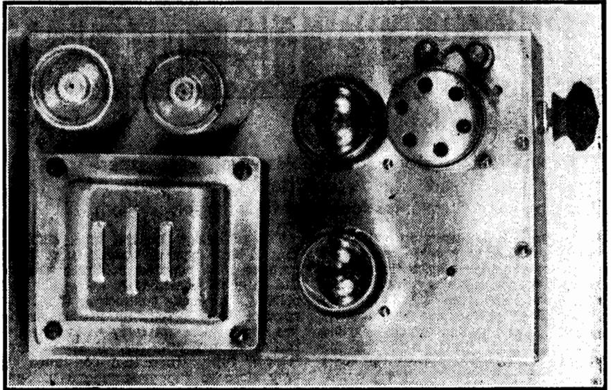
Here is a picture of the amplifier showing the layout of the parts.
