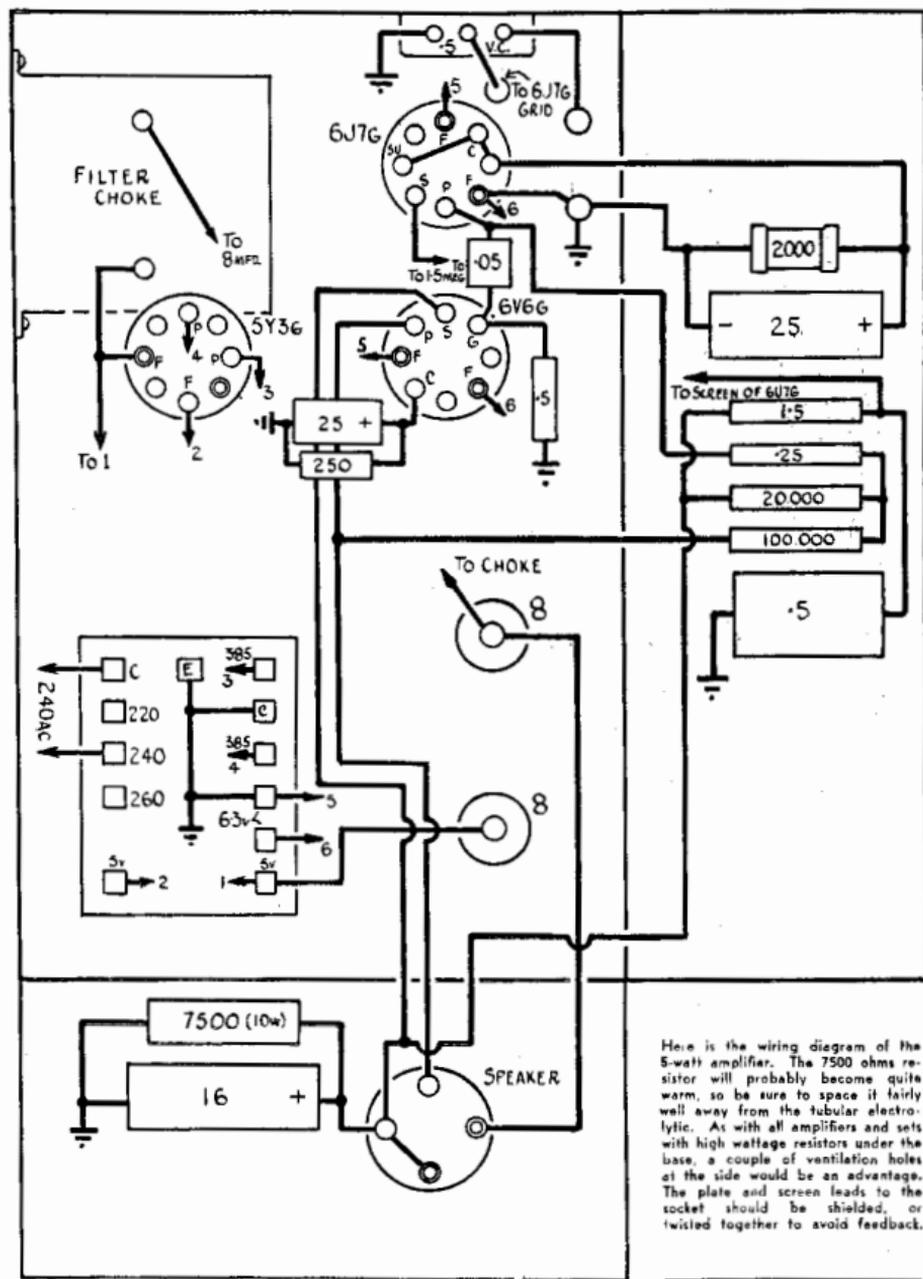
Here is the wiring diagram of the 5-watt amplifier. The 7500 ohms resistor will probably become quite warm, so be sure to space it fairly well away from the tubular electrolytic. As with all amplifiers and sets with high wattage resistors under the base, a couple of ventilation holes at the side would be an advantage. The plate and screen leads to the socket should be shielded, or twisted together to avoid feedback.
