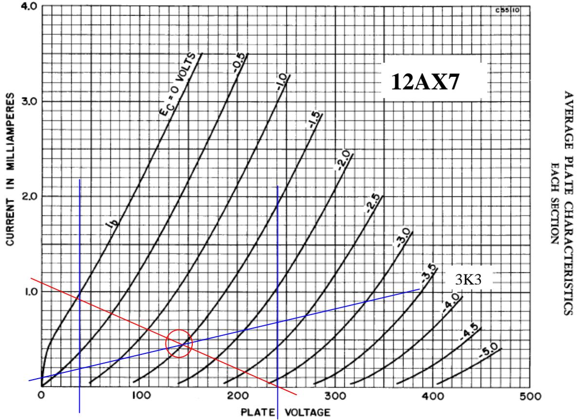
PI 12AX7 V2B: VS2=250V; Va=205V; Vc=95V; Rk=2k2; Vk=0.88V; Ia=0.4mA; RLdc=100 + 235k. Max voltage swing about +45V for anode to rail, and Vak can swing -80V from 110V at idle down to about 30V. Perhaps increase bias current a bit by reducing 2k2 to 1k8.
