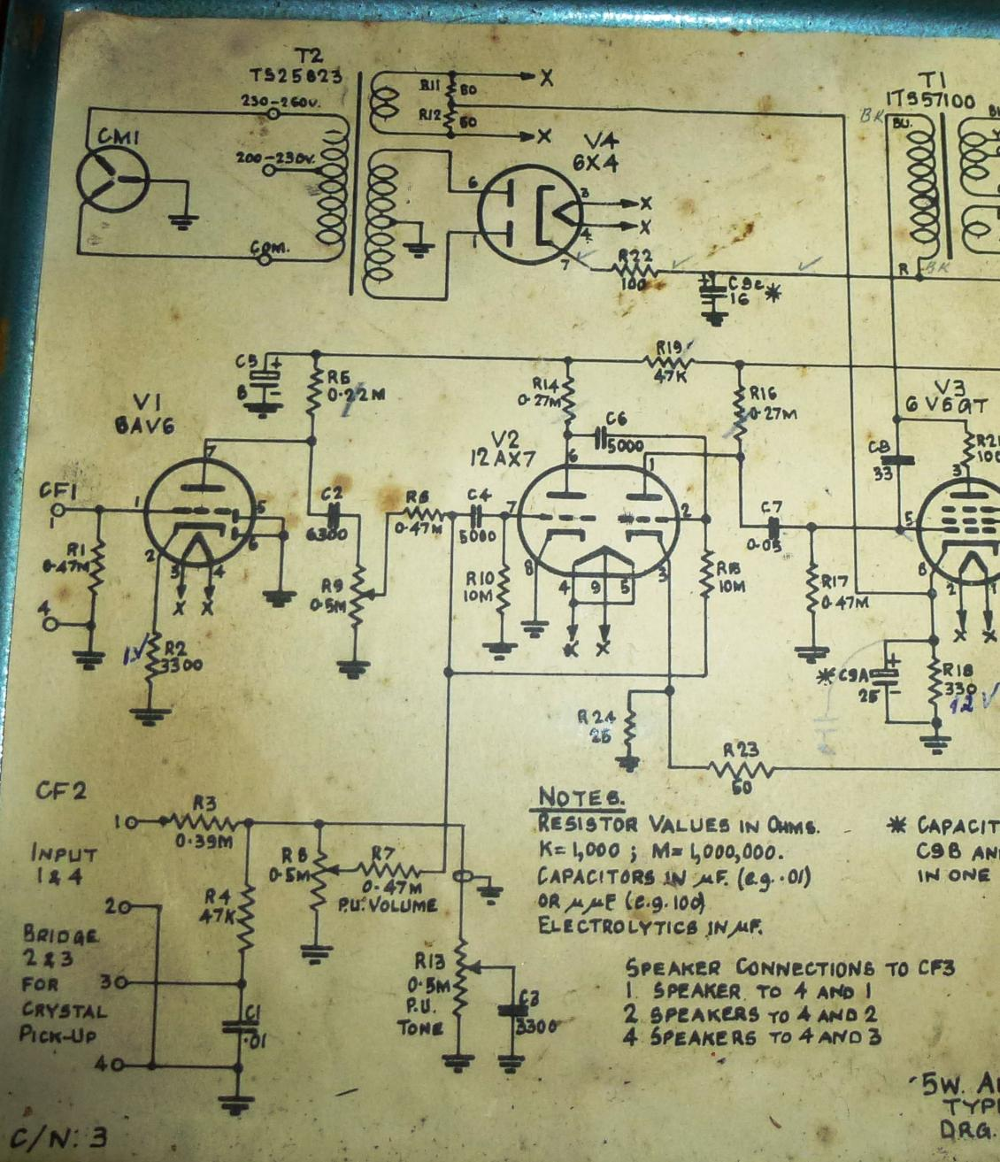
CF3 BK. 01. 600 BK 02. 300 A BLUE 03 1500 04. COM. GR FLLOU W. ORANI 1 R20 22K 610 100 SR21 C98# + \* CAPACITORS COA, COB AND COC ARE IN ONE ASSEMBLY. SW. AMPLIFIE TYPE 056806. DRG. 5680601.
