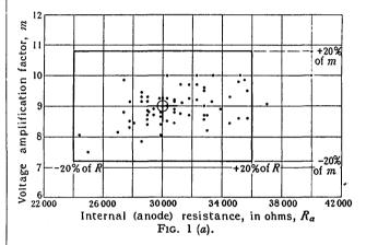
In selecting lamps for life-test it is the practice to subject a large number to a candle-power rating test, and, from this large number, to select for life-test a comparatively small number, the candle-power ratings of which lie within the narrow central zone of the total spread shown by the large number. The average life of this small number which is life-tested, is, of course, much more truly representative of the average life of the factory product than would be the average life of a
