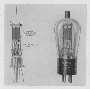
Fig. 10-No. 262A mount and completed tube.
