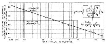
Fig. 9—Fundamental disturbance output current as a function of the grid-to-heater resistance.
