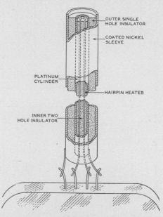
Fig. 6—Experimental heater arrangement for the study of the magnetic effect.
