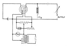
Fig. 4—Circuit for the study of the electrostatic effect in the presence of large disturbance outputs due to the magnetic field.
