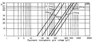
Fig. 3-Cumulative distribution characteristics of EF86 valves
