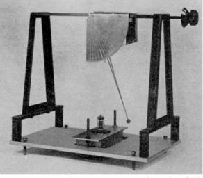
Fig. 6—Apparatus for measuring microphony by shock excitation
