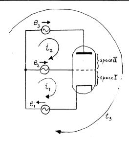
Fig. 2.—Basic triode circuit treating the valve as  $\alpha$  passive circuit element.  $i_1$ ,  $i_2$  and  $i_3$  are mesh currents, and  $e_1$ ,  $e_2$  and  $e_3$  are ideal zero impedance small-signal generators.
