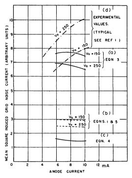
Fig. 1.—Values of induced grid noise: (a) Calculated on the theory of references 3, 4 and 5; (b) Calculated on the theory of reference 1 with theoretical values of ct; (c) Calculated on the theory of reference 2; (d) Typical experimental values. (Reference 1.)
