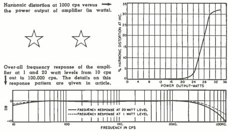
The available power of the amplifier before the clipping action and the over-all power of the unit at one per-cent harmonic distortion.
