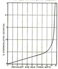
(60 to 6000 cps mixed 4:1 at 20 watts) is 1.3% while the mid-band harmonic distortion at 20 watts is .3%. The damping factor is 7:1 and the inverse feedback 14 db. Taps are provided for 4, 8, and 16 ohm speakers.
